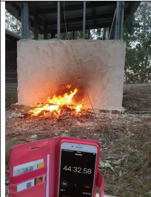
Photo 21: Fire 44 min 32 sec into 60-minute test
