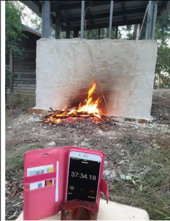
Photo 19: Fire 37 min 34 sec into 60-minute test
