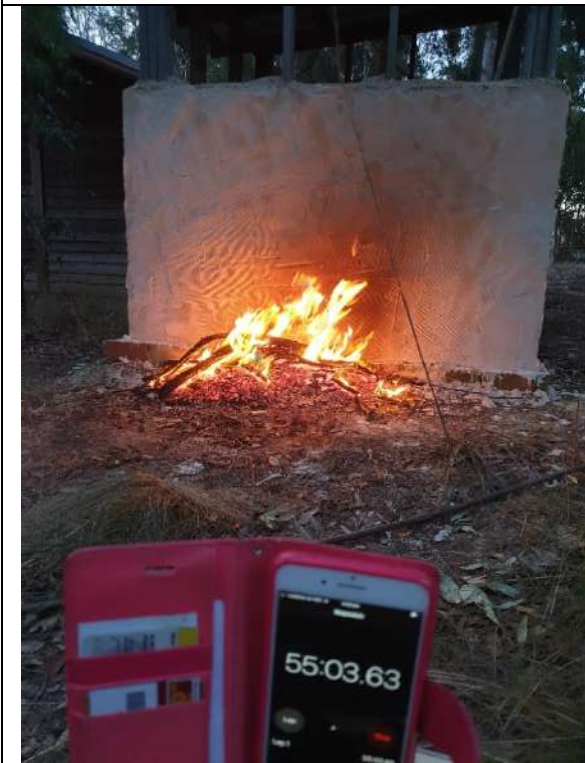
Photo 23: Fire 55 min 03 sec into 60-minute test
