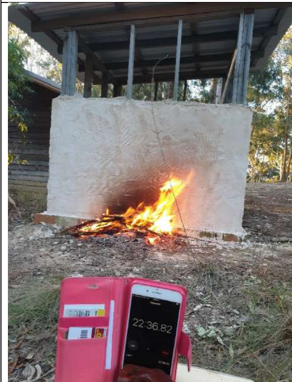
Photo 13: Fire 22 min 36 sec into 60-minute test
