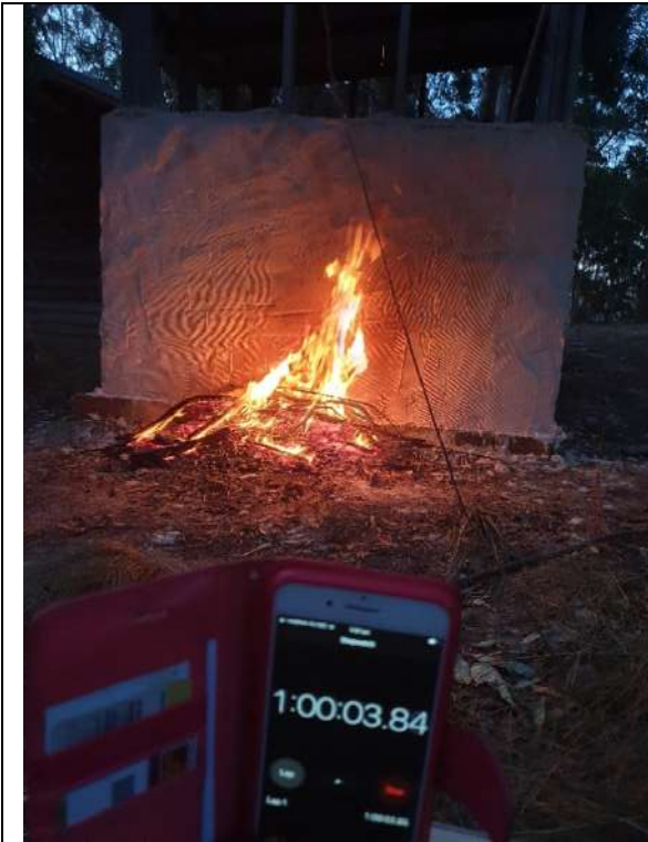
Photo 25: Fire 1 hour into 60-minute test
