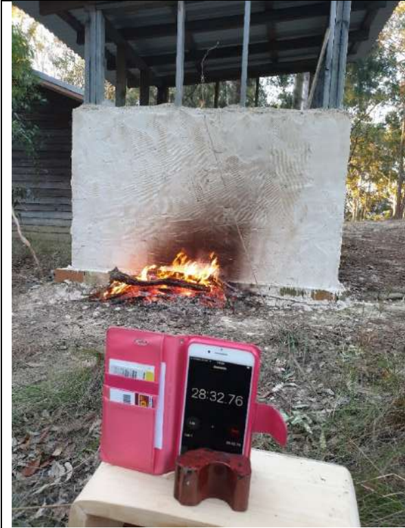
Photo 15: Fire 28 min 32 sec into 60-minute test
