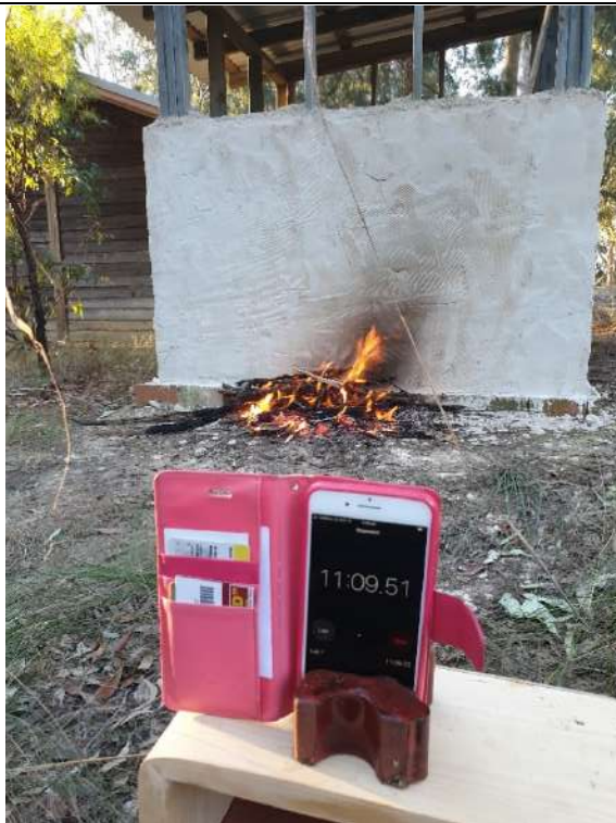
Photo 9: Fire 11 min 9 sec into 60-minute test
