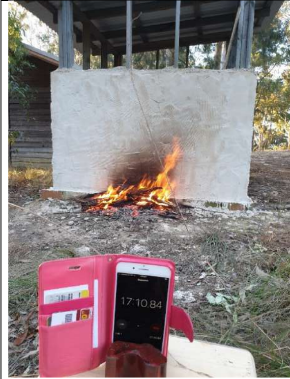
Photo 11: Fire 17 min 10 sec into 60-minute test
