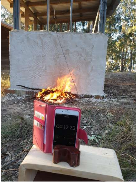
Photo 7: Fire 4 Min 17 sec into 60-minute test
